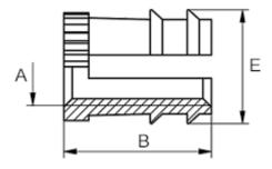
Female thread A = M3,5 Length B = 5.0Max outer diameter E = 6.00Number of cramping feathers = 1
